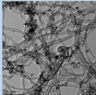
Example of a cobalt catalyst supported on Carbon Nanotubes (Rose *et al.*, 2014)
