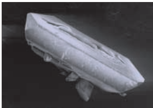
Crystal of struvite precipitated from sludge liquors (Doyle et al, 2000)
