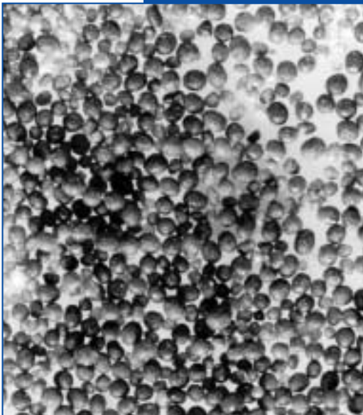
Recycled phosphates recovered from sewage and ready for industrial use (magnified)
