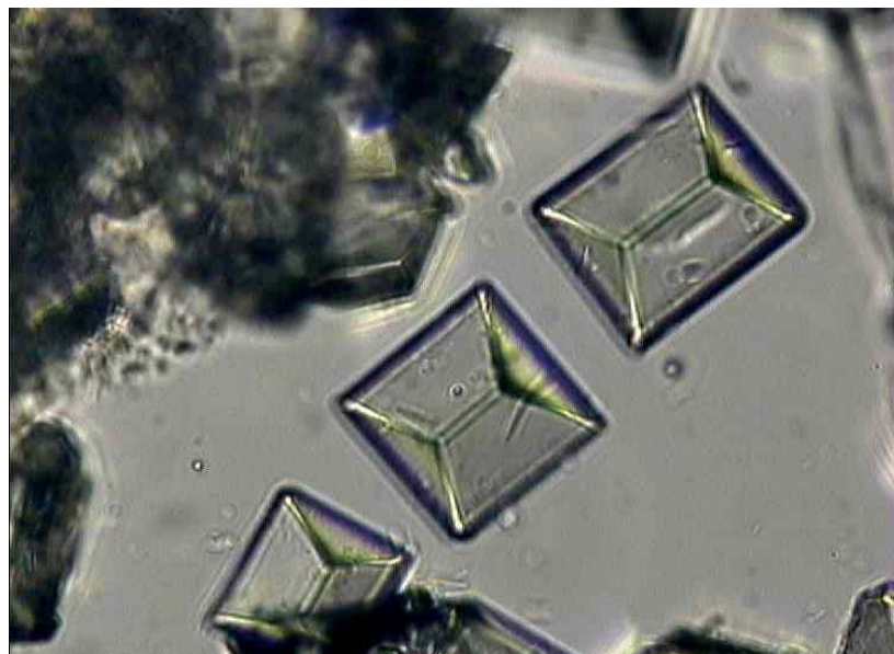
Fig. 12. Regular orthorhombic crystals structure of precipitated struvit using magnesium sulphate
